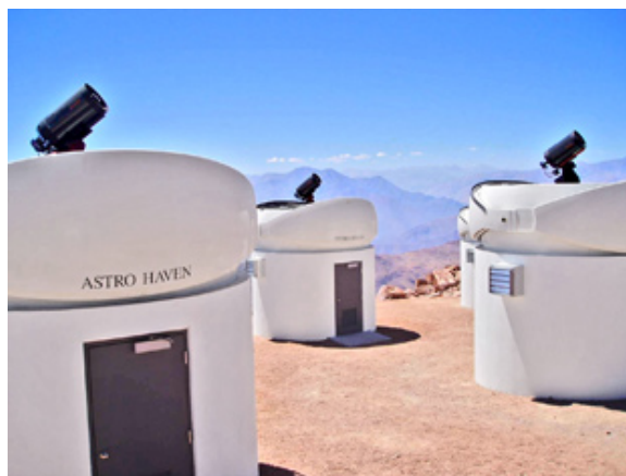
From left to right, the PROMPT-5, -3 and -2 telescopes. We have been using three 0.36-meter Schmidt-Cassegrain telescopes from Celestron while our final optics are being prepared. In September 2005, we will upgrade to six 0.41-meter Ritchey-Chrétien telescopes by RC Optical Systems.
